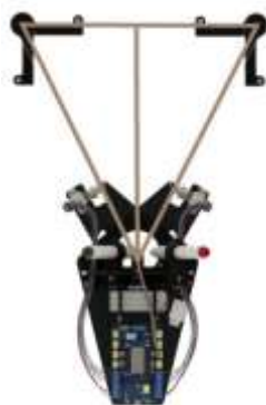
Figure 9. Drawing robot positioning using anchored strings
