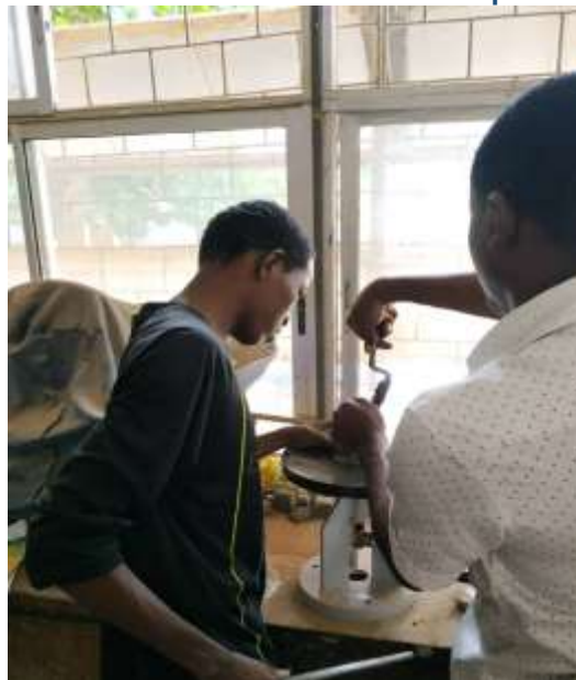
Figure 5 - Determination of Consistency
