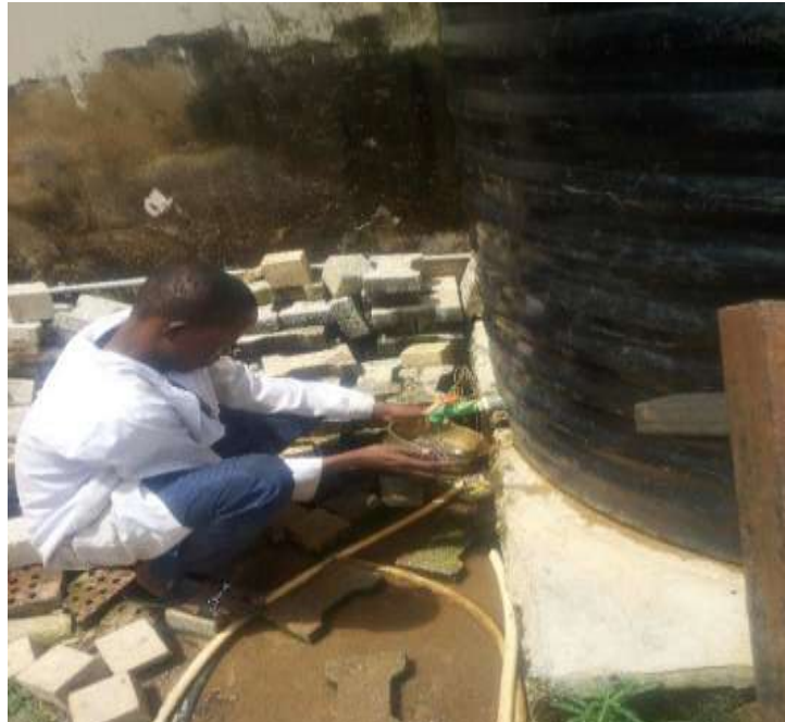
Figure 2 - Determination of GHA Fineness by fineness test
