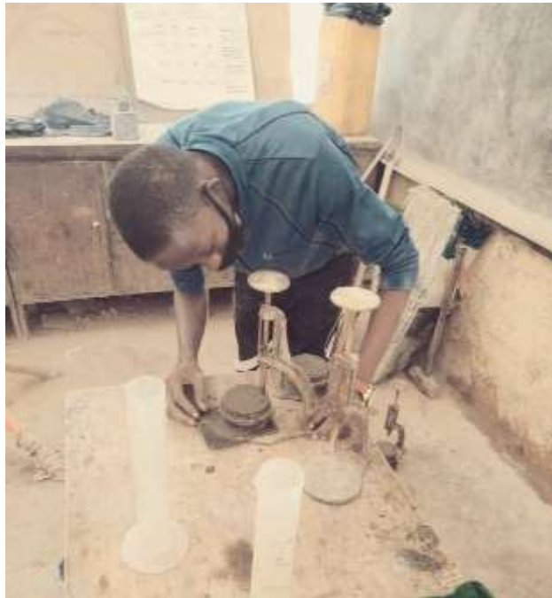
Figure 6 – Determination of Setting time
