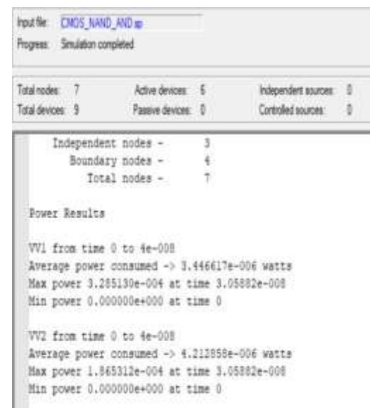
Fig. 7. Power utilization of Basic CMOS NAND Logic.
