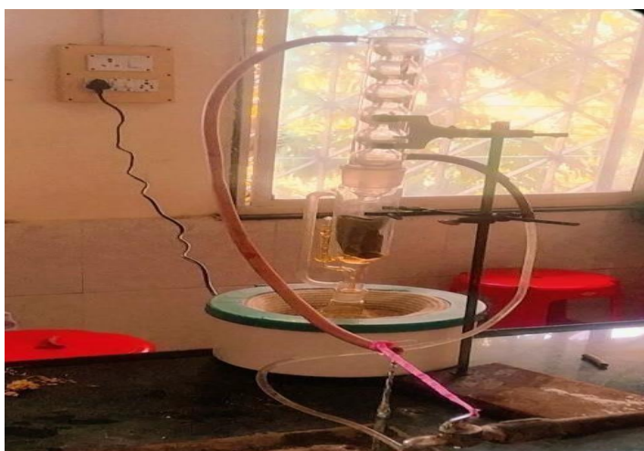
Fig No 5: - Extraction process by Soxhlet Apparatus
