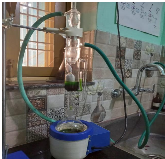
Fig 2 Soxhlet Apparatus for steam distillation
