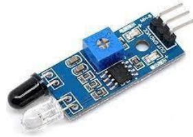
Fig 4. IR Proximity Sensor
