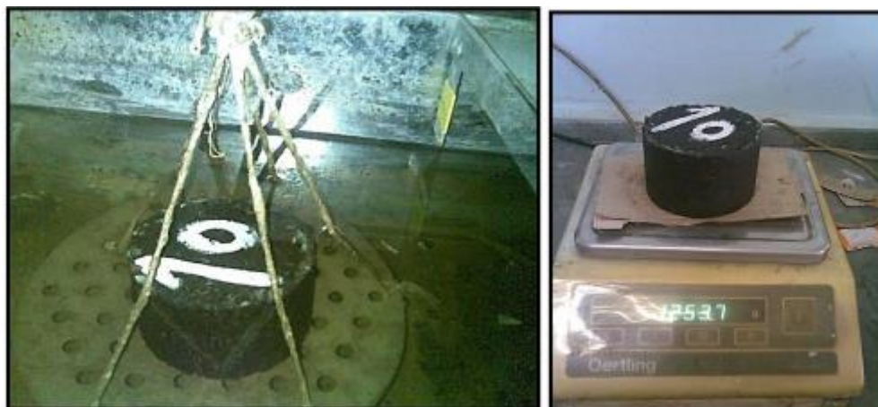
Figure 7. Weighing asphalt samples in air and water
