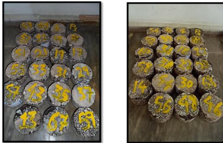
Figure 6. Preparing the cores in 2 saturated and dry states
