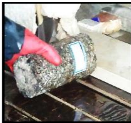
Figure 5. Cutting the cores
