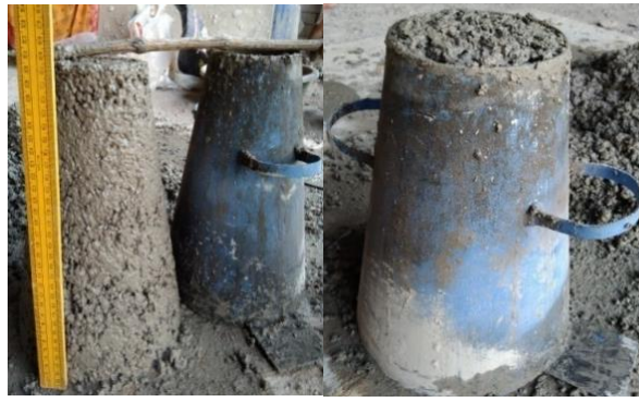
Fig 1: - zero slump concrete mix
