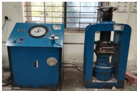
Figure 3: - Compressive strength test
