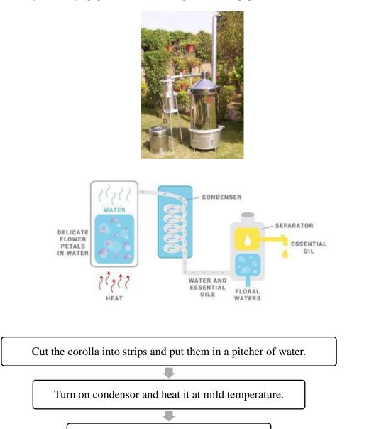
Collect the distillate into a recipient flask.
