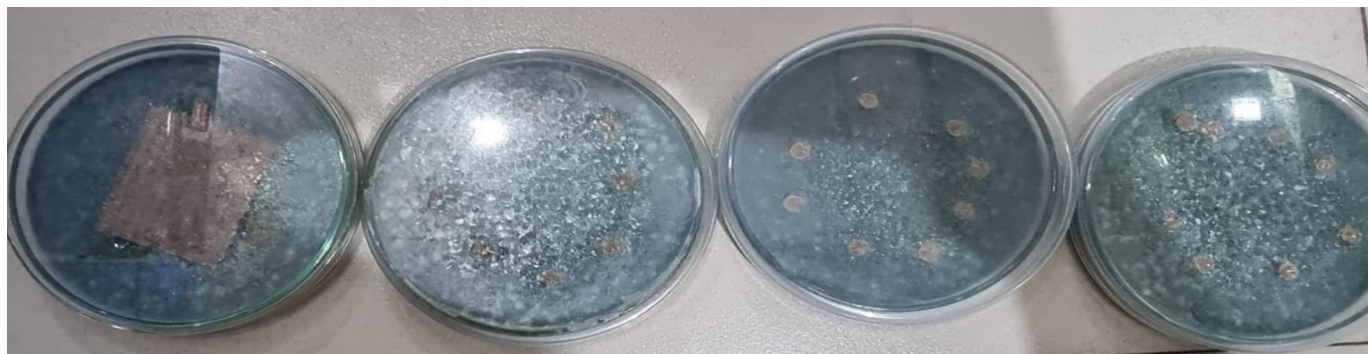
Fig. 2: Antifungal effect on uncoated and coated corrugated sheets on day 5 of observation.
