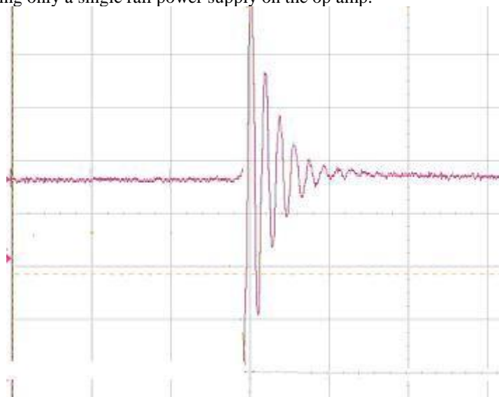
Figure 4: Care must be taken when using single rail op amps since shock can cause negative voltage spike ringing that can damage op-amp inputs if not squelched.
