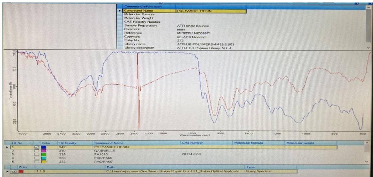
Figure 4. ATR-FTIR library indicating presence of polyamide microplastic in the gut sample of said fish
