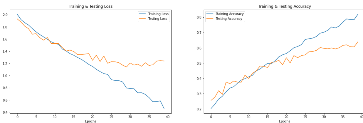
Fig.3: CNN Model Loss and Accuracy plot against epochs for Training and Testing Data
