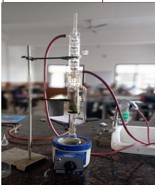
Figure 1. exteration of Lantana Camera by Soxhlet Appratus
