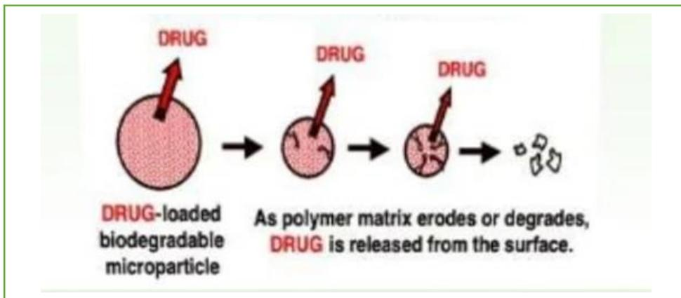
**Fig. No. 3- Drug released by polymers by degradation.**
