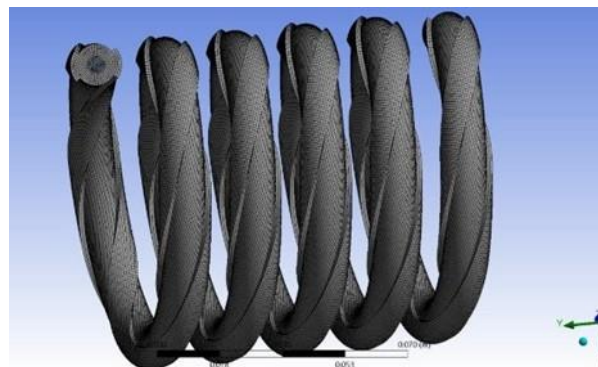
Fig. 5 Meshing of 2 ribs and 10 revolutions
