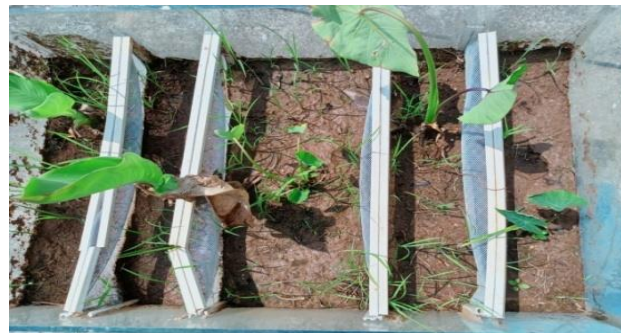
Figure 1 Vertical Constructed wetland planted with Canna generalis and Hedychium Coronarium
