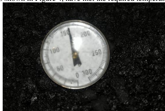
Figure 4 Measurement of Asphalt Mixture Temperature Above Dump Truck
