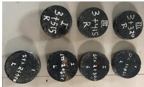
Figure 10. Sample of Sand Sheet By Core Drill
