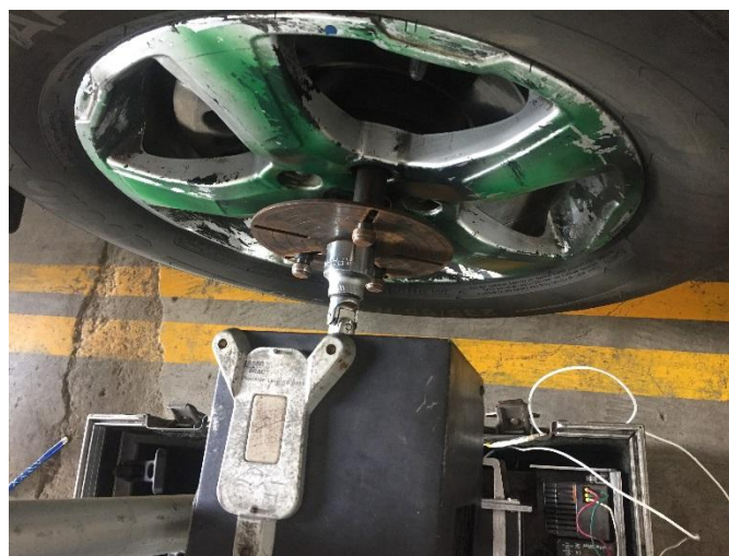
Figure 3. Wheel drive adaptor with fixture plate
