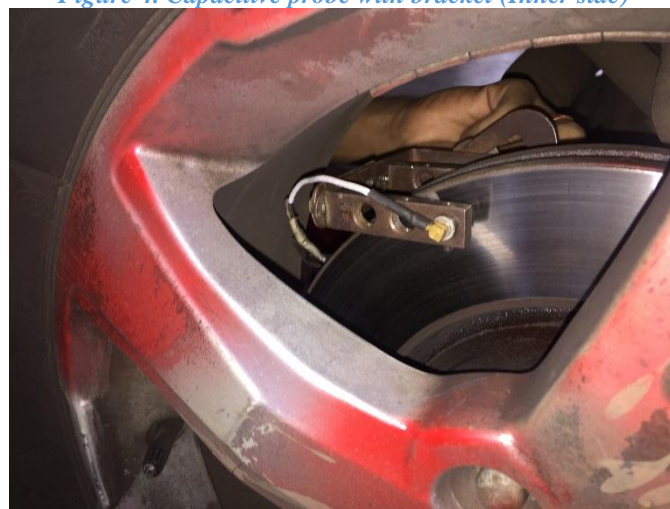
Figure 5. Capacitive probe with bracket (outer side)
