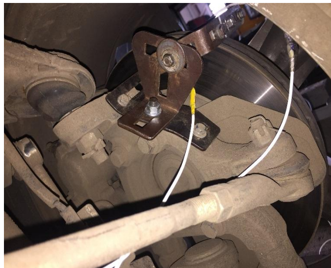
Figure 4. Capacitive probe with bracket (Inner side)
