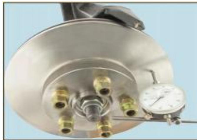
Figure 7. Dial Indicator with Brake Disc
