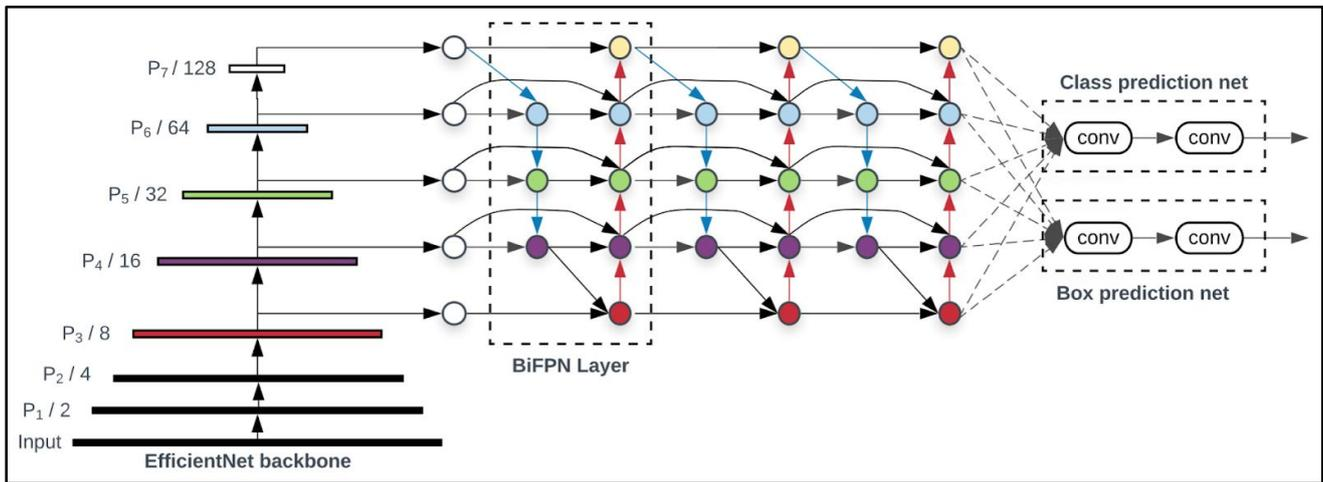
Backbone network: Same width/depth scaling coefficients of EfficientNet-B0 to B6 are used so that ImageNet pre-trained checkpoints can be used.
