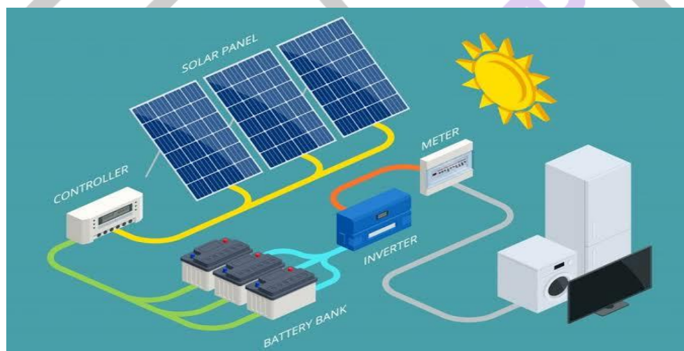
Fig.4 Solar Energy Generation System
