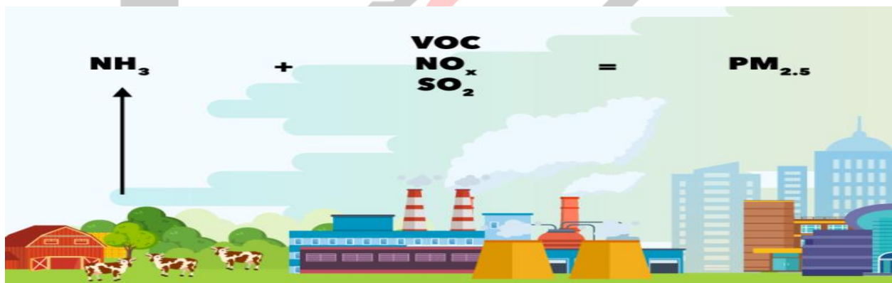
Figure 2. Ammonia ( \text{NH}_3 ) can combine with volatile organic compounds (VOC), nitrogen oxides ( \text{NO}_x ) and sulfur dioxide in the air to form health-harming small particles ( \text{PM}_{2.5} ).
