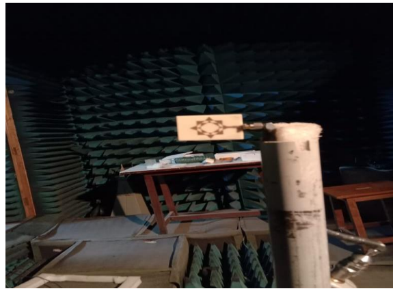
Fig 17 Front View of Fractal Antenna in Anionic Chamber
