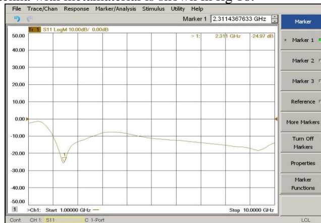
Fig 19 Measured Return loss of Fractal Antenna
