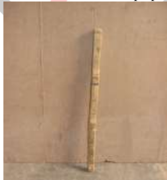
Figure 4. 5 Bamboo Sample (In Natural Condition) for Pullout Test.
