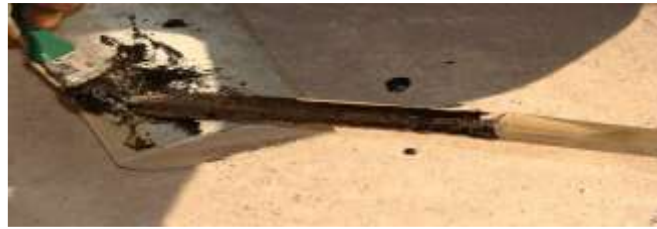
Figure 4. 6 Bamboo Sample Coated with Tar
