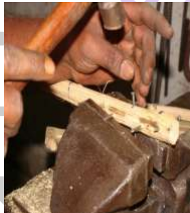
Figure 4. 8 Hammering the Nails through the Holes,
