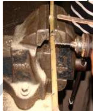
Figure 4. 7 Making Hole by Using Drill Machine,
