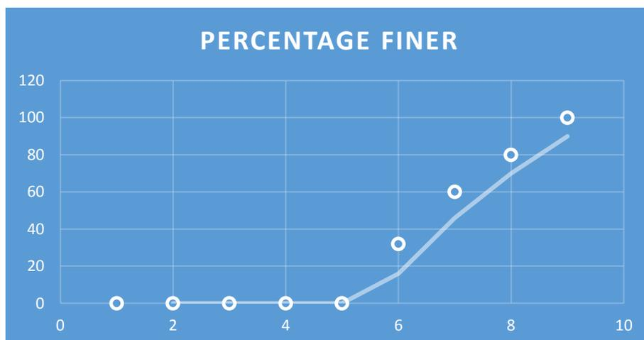
**Fig. 5:** Particle Size distribution graph for Sample B
