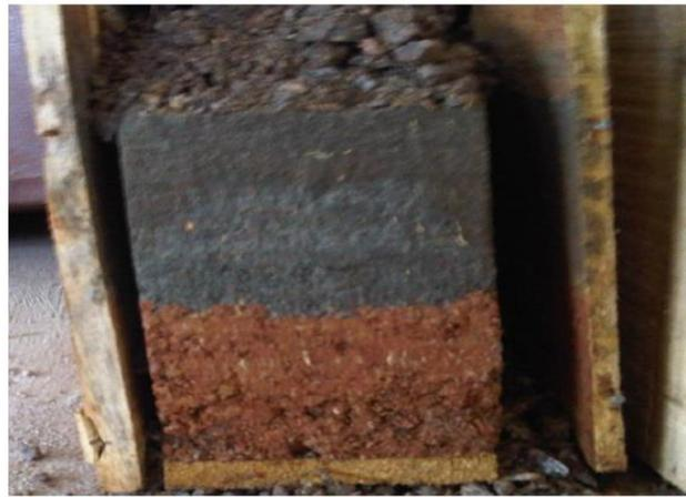
**Fig. 9:** Plate 8 – Merging - Improper Separation of sub-grade from the sub-base
