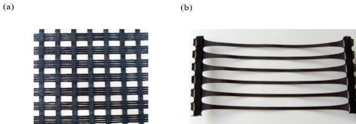
Fig. 2: (a) Biaxial woven geogrid and (b) Uniaxial geogrid
