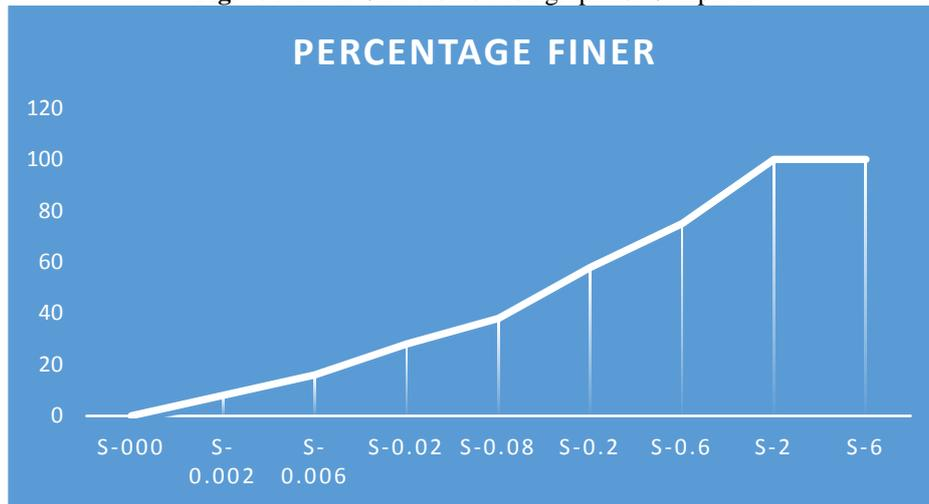
**Fig. 6:** Particle Size distribution for Sample C
