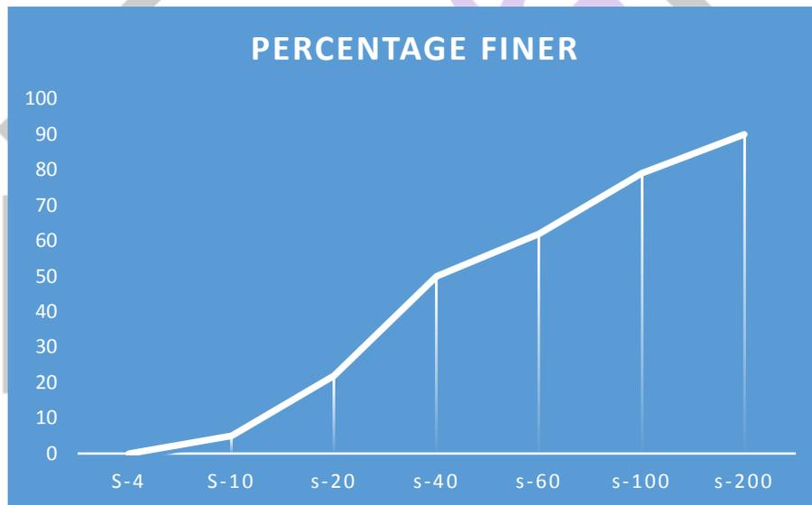
**Fig. 4:** Particle size distribution graph for Sample A
