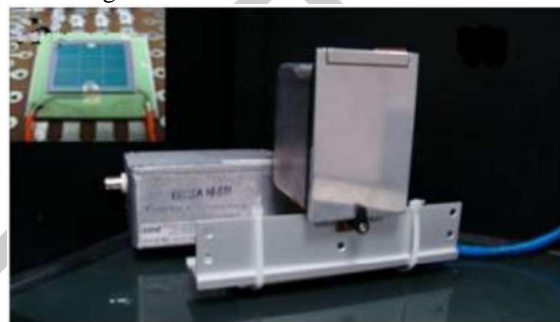
Fig. 5: The vacuum chamber used in this work and the PIN diode (inset)
