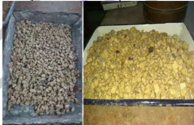
Fig. 1: Crushed RBWA of size 10mm and 20mm
