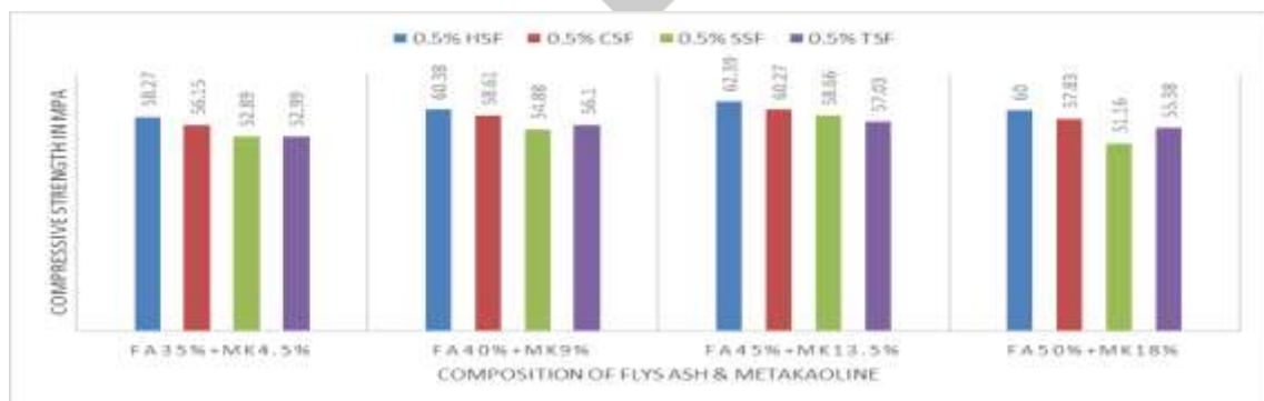
Fig 8: Compressive strength results for concrete mixes composed of various substitutions of FA+MK reinforced with 0.5% HSF, CSF, SSF & TSF
