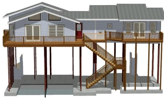
Figure 1. 2 Elevation on piers
