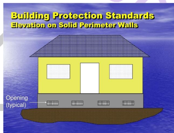
Figure 1.1 Elevation on solid perimeter foundation walls
