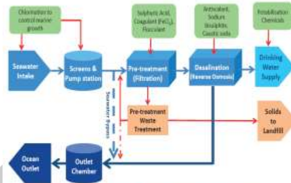
Fig:2- RO Desalination process (Source: Fichtner, 2011)
