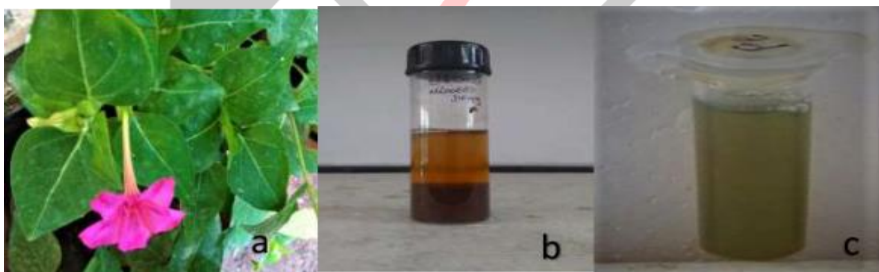
Figure 1: a) Mirabilis jalapa plant with flower b) Mirabilis jalapa fresh flower extract c) Mixture of Mirabilis jalapa flower extract and iron sulphate over 2 hours incubation.
