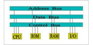
So an embedded system has a micro-processor or micro controller for processing information, memory for storing embedded software programs and data and I/O interfaces for external interfaces. The functional diagram is given above.
