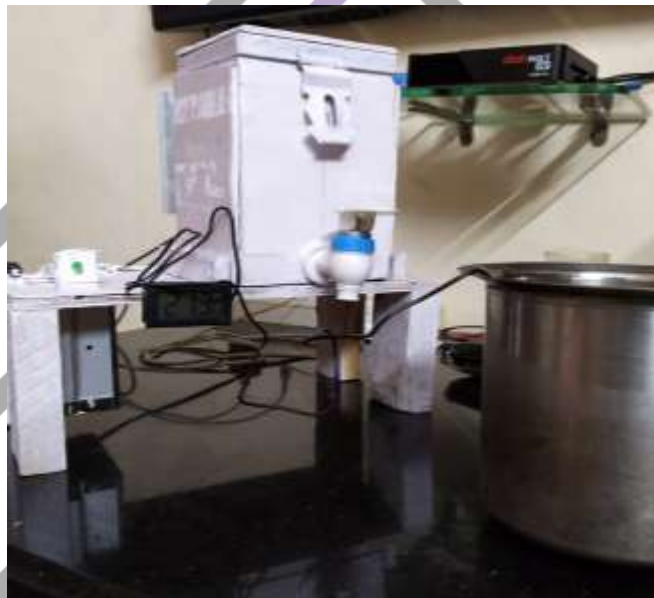
Figure 2: Experimental Representation of Thermoelectric Water Cooler.
