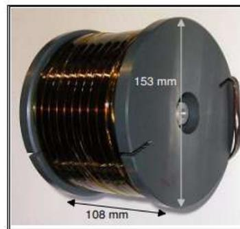
**Inductor specification and physical 'as-built' configuration**
