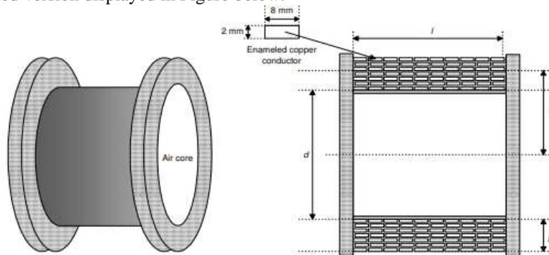
**Inductor design using flanged air core former and enameled copper conductors**
