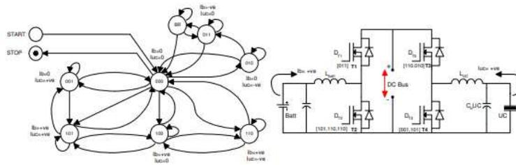
**Active switches of the converter in relation to the active states of the PES State machine**
