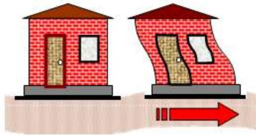
Figure Effect of Inertia on Building
