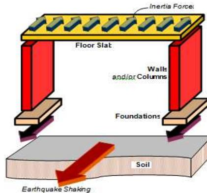
Figure Final transfer of seismic inertial forces to the structural components
