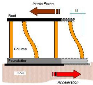
Figure Effects of Seismic Inertial Force on the Relative Motion of the Structure
