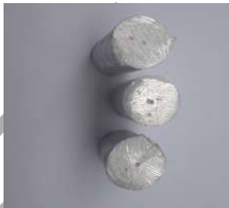
Fig 7: specimen for hardness testing.
