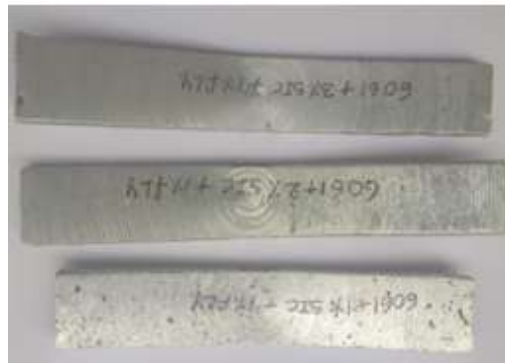
Fig 5: flexural testing specimen.
