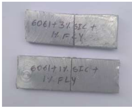
Fig 6: specimen for impact testing.
