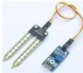
Figure 4. Soil Moisture Sensor
