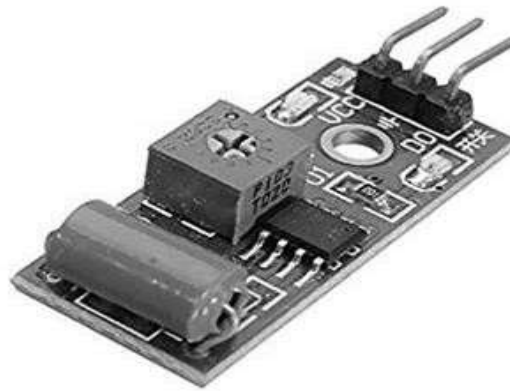
Fig 2. Vibration sensor or Motion Sensor
