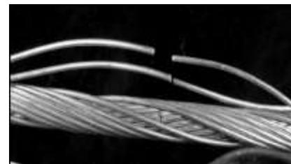
Fig 1. (c) Spicing and broken strands
