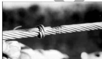
Fig 1. (b) Worn-out due to broken tie wires
