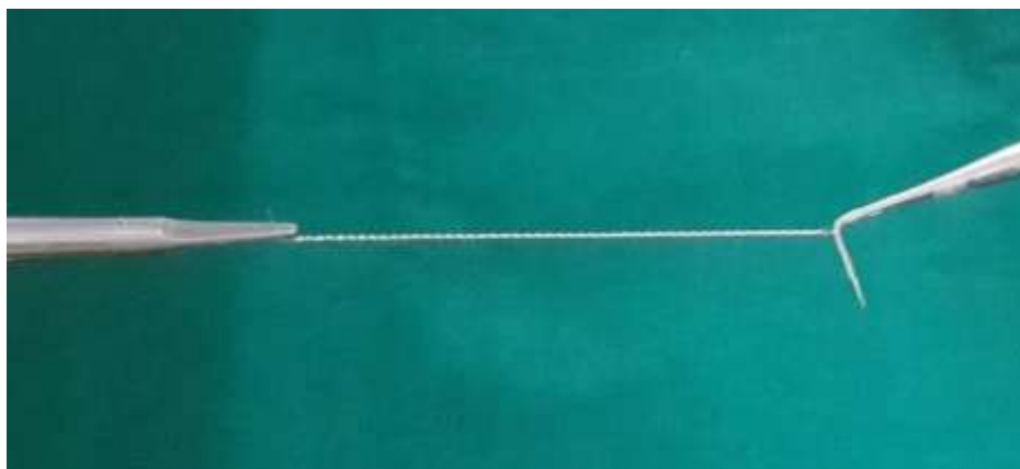
Custom made twisted wire (0.010" Stainless Steel Ligature{ HP Company})
