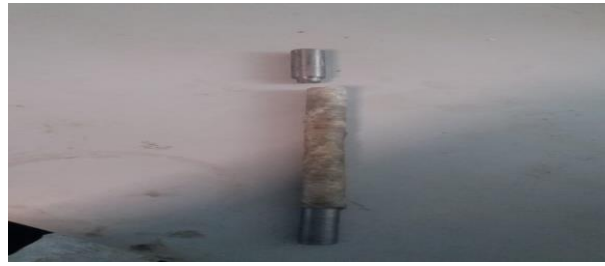
Fig.11 Carbon Fiber Shaft after test
