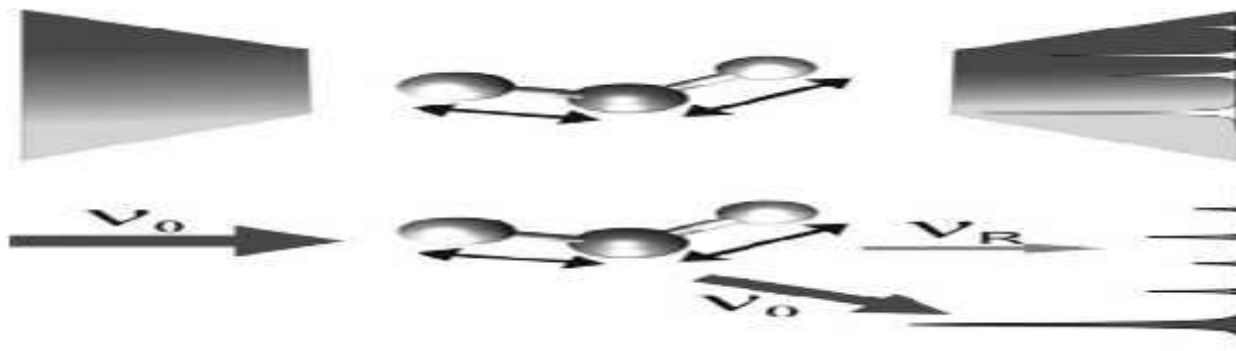
Figure 1. Illustration of the excitation of molecular vibrations in IR (top) and Raman (bottom) spectroscopy.
