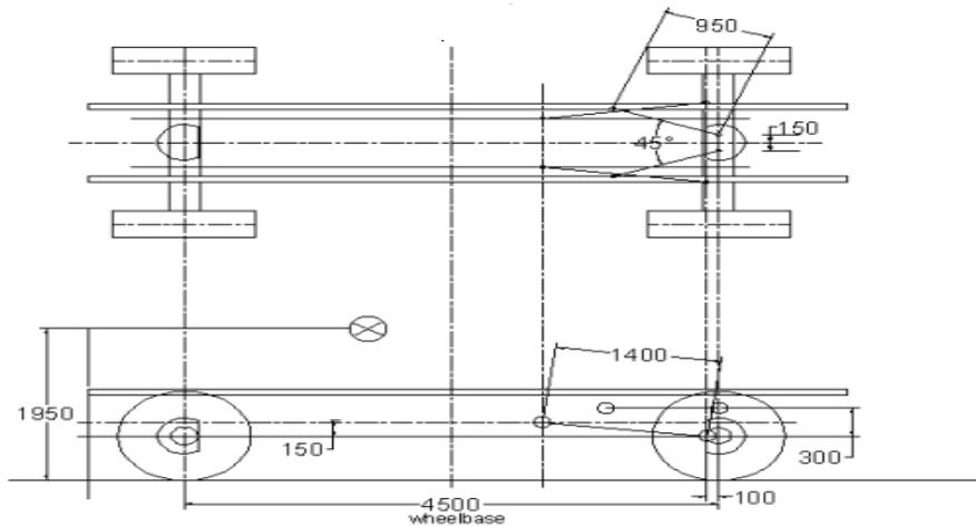
Locations of lower and upper links in between rear axle and chassis in multi-link suspension system as per research available on locating links without compromising its mobility and excellent vehicle stabilizing features of multi-link suspension.
