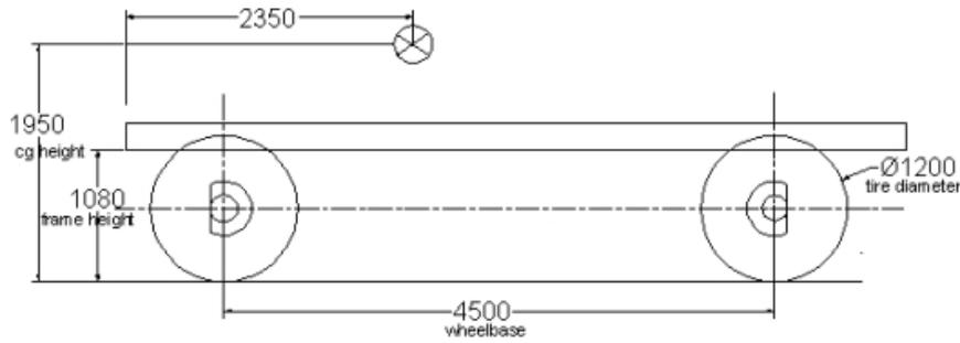
The first step in building a four-link consist of taking dimensions from Workshop Maintenance manual and constructing diagram in AutoCAD. By using this figured out, the axle centerline points on the bottom half were located, where the frame should sit above the axle. The center of gravity of the sprung weight was located.
