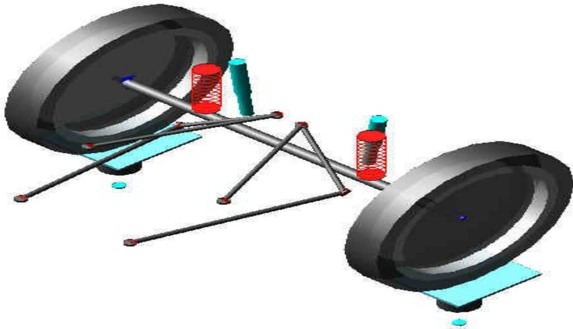
Multi body simulation of Multi-link rear suspension system using MSC ADAMS/CAR
