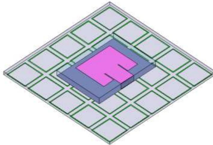
Figure 6 Microstrip Patch Antenna with FSS Substrate
