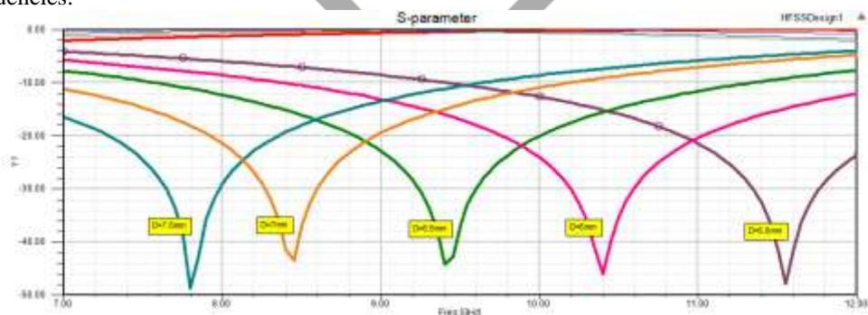
Figure 5 Transmission Coefficient of Unit Cell for Various Loop Dimensions
