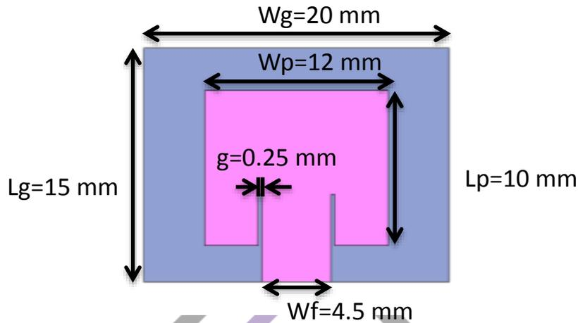
Figure 1 Dimensions of the designed antenna
