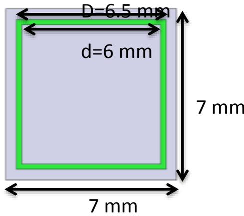
Figure 3 Top view of the unit cell
