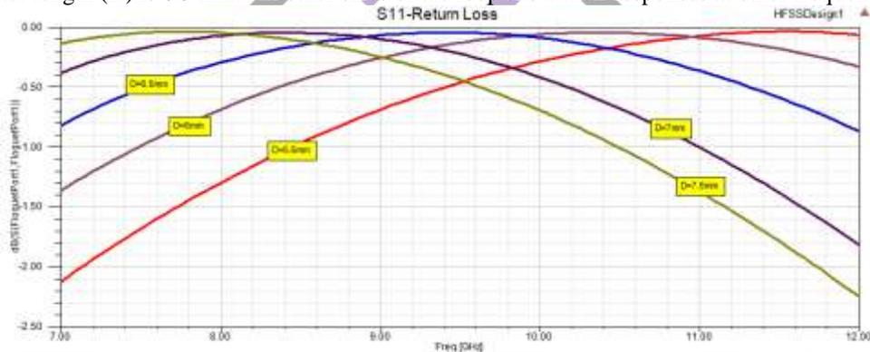
Figure 4 Reflection coefficient of Unit Cell for various loop dimensions
