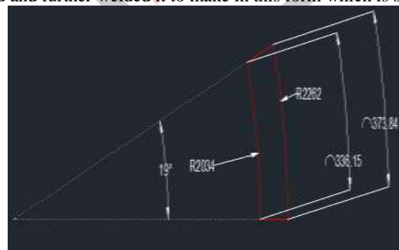
Surface Development of Combustion Chamber
