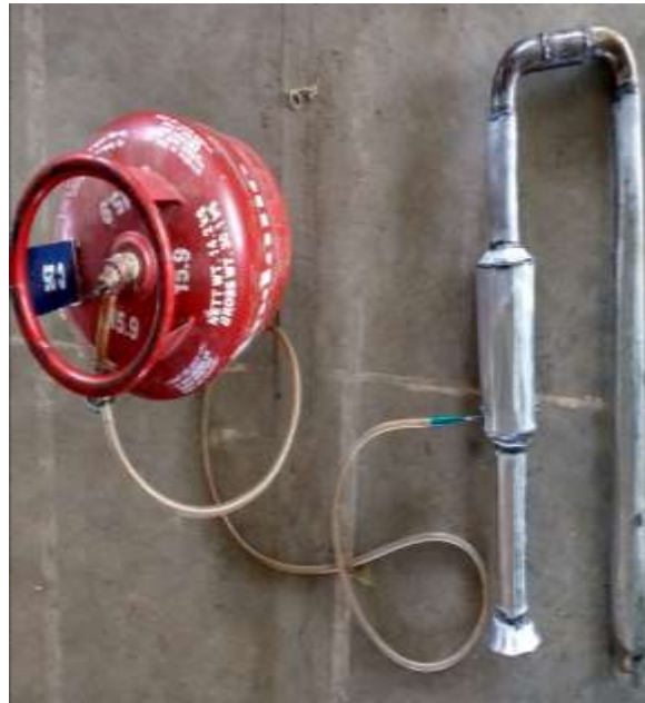
Assembled Valveless Pulsejet Engine with gas Cylinder
