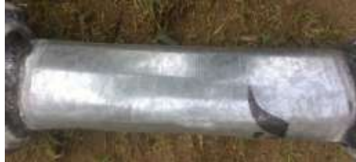
Fabricated Intake Tapered Section
