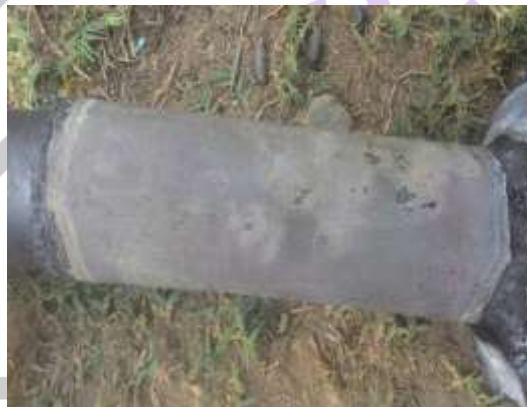
Fabricated component joining Combustion Chamber and U-Section
