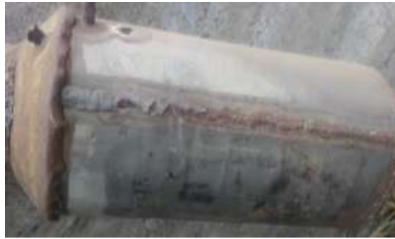
Fabricated Combustion Chamber
