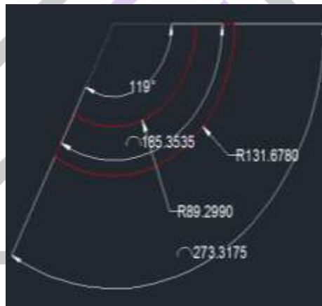
Surface Development of Inlet Nozzle
