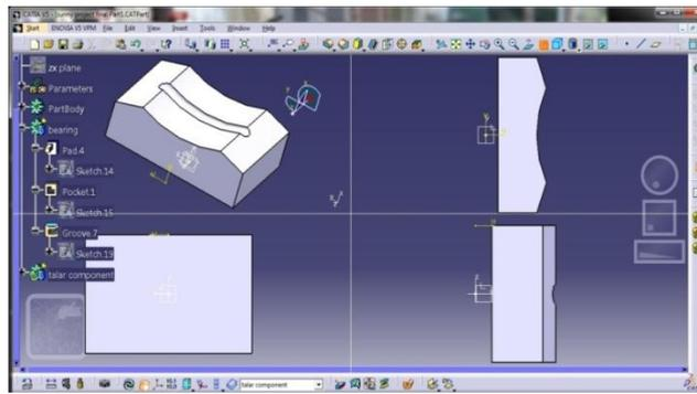
Fig.6 Design of mobile bearing component
