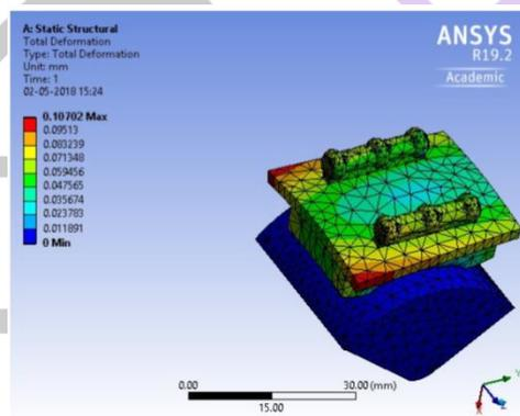
Fig.12 Total deformation of Ti-6Al-4V Material
