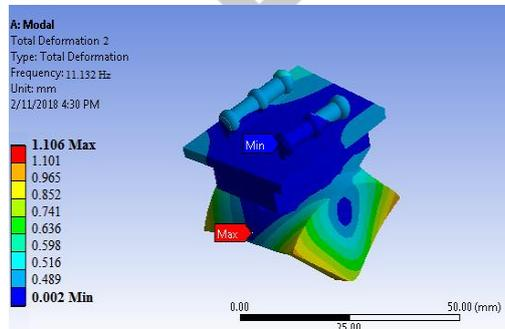
Fig.17 Modal analysis of Ti-13Nb-13Zr Material
