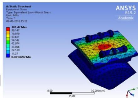
Fig.11 Von-mises stress of Ti-6Al-4V Material
