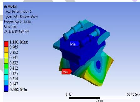
Fig.16 Modal analysis of Ti-6Al-4V Material
