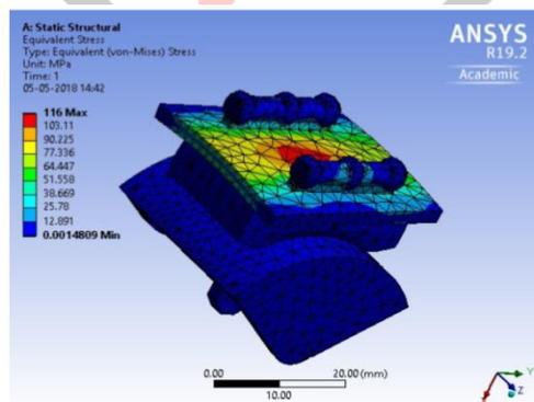
Fig.9 Von-mises stress of Co-Cr-Mo Material
