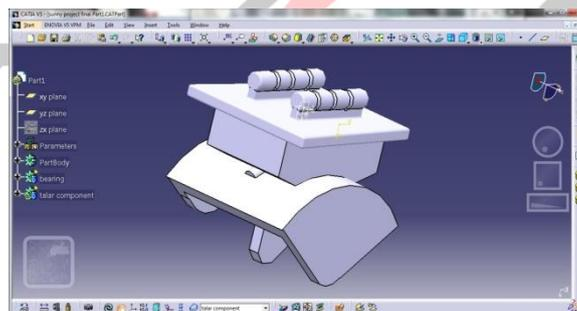
Fig.8 Assembly of ankle joint implant
