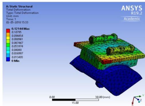
Fig.14 Total deformation of Ti-13Nb-13Zr Material
