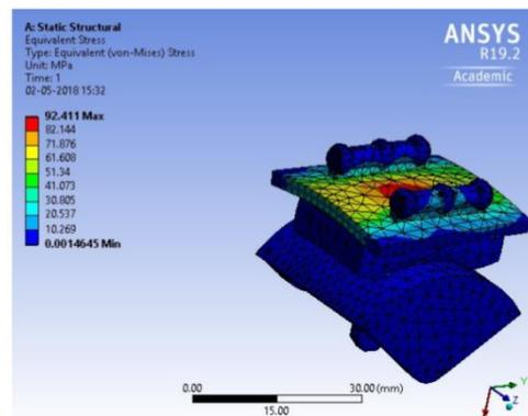
Fig.13 Von-mises stress of Ti-13Nb-13Zr Material
