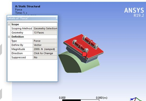
Fig.8 Loads and Boundary conditions
