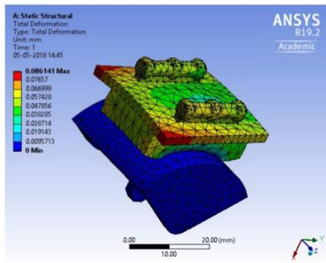
Fig.10 Total deformation of Co-Cr-Mo Material
