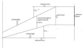
Fig.1.2 conceptual sketch of aircraft wing
