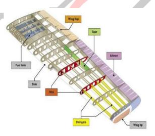
Fig. 1.1 simple aircraft wing structure
