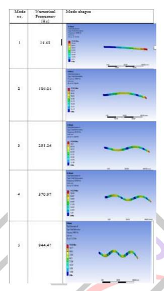
Table. 7.4 Cantilever beam numerical frequency with its respective mode shapes
