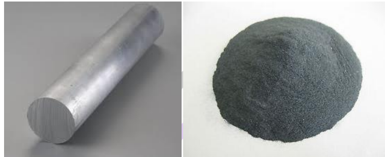
Figure 3 Aluminum Matrix Material & Silicon Carbide (SiC) Powder
