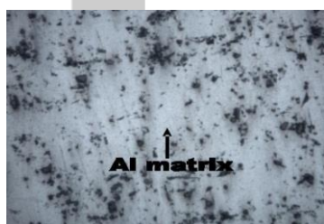
Figure 8 & 9 Microstructure of 14 & 28 wt. % silicon carbide (SiC) reinforced Aluminum matrix composites (AMC)
