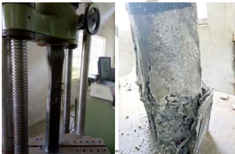
* Failure of long column specimens at the ends
