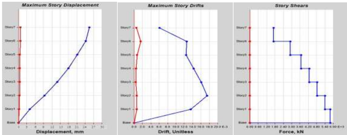
Fig-4.8: Storey Displacement, Storey Drift, Base Shear
