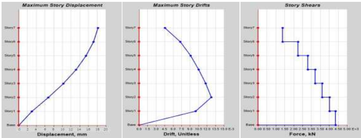
Fig-4.2: Storey Displacement, Storey Drifts, Base Shear.
